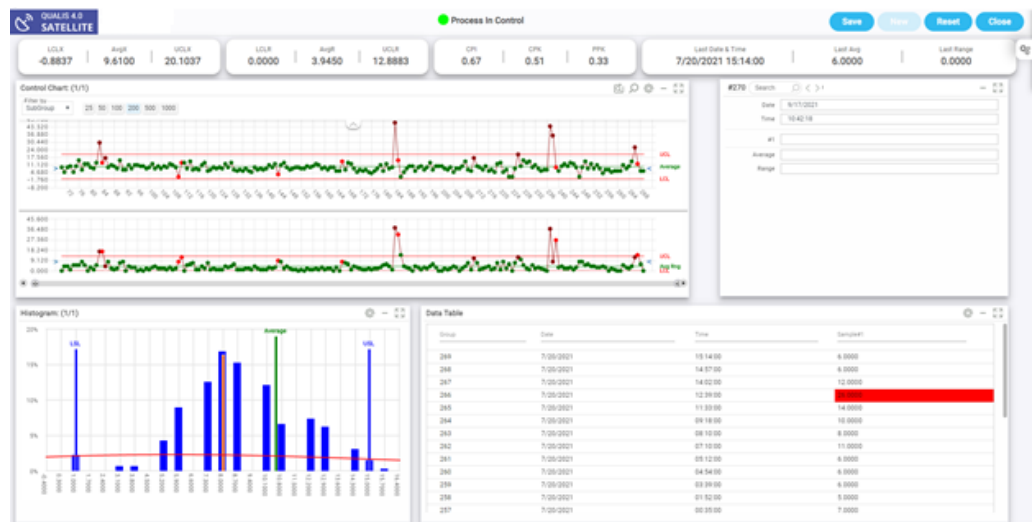
Figure 2: Change over data of machine Y in a real-time control chart
