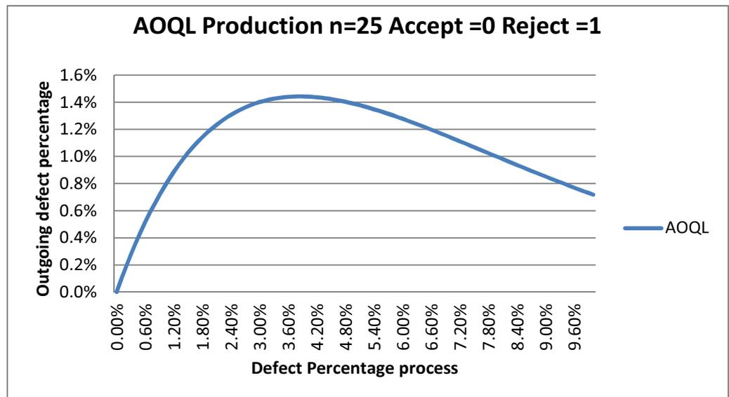
Figure 2: Average outgoing quality for a specific defect percentage
